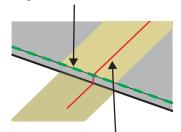
The detected strip edge position value is compensated according to the pass line position of the strip as measured by the laser.
