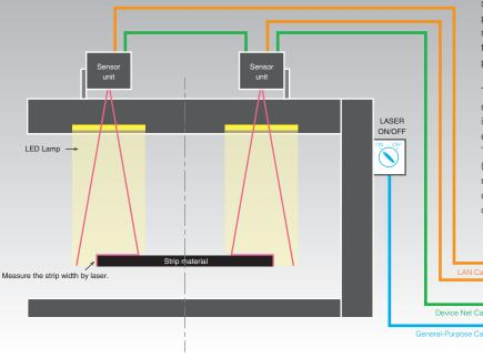
The system consists of LED light source for illumination, Sensor unit for detection of the strip and a specialize control panel with image processing unit for data analysis and I/O management. The sensor unit is connected to the specialize control panel using general purpose device net cable and LAN cable
