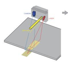
The strip is illuminated using LED and the edge position is determined by using the average value.
